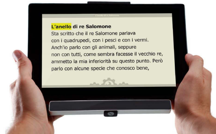
Figure 2: The current prototype (left) is composed of a wood stand that holds a 10" tablet and an eye tracker. In future refinements of the prototype we will aim at integrating the eye tracker on the tablet itself (as seen on the mock-up on the right).
